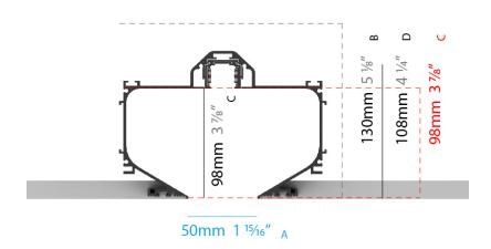
A: OPENING WIDTH B: RECESS DEPTH C: OPENING DEPTH D: PROFILE HEIGHT E: WIDTH INCLUDING MOUNTING BRACKETS
