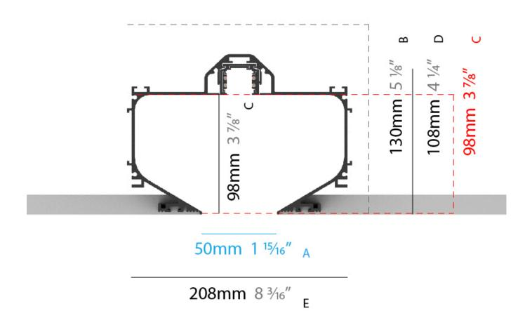
A: OPENING WIDTH B: RECESS DEPTH C: OPENING DEPTH
