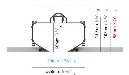
A: OPENING WIDTH B: RECESS DEPTH C: OPENING DEPTH D: PROFILE HEIGHT E: WIDTH INCLUDING MOUNTING BRACKETS
