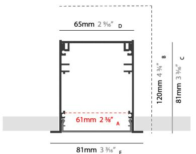
A: OPENING WIDTH B: RECESS DEPTH C: PROFILE HEIGHT D: PROFILE WIDTH E: MOUNTING INCLUDING FLANGE
